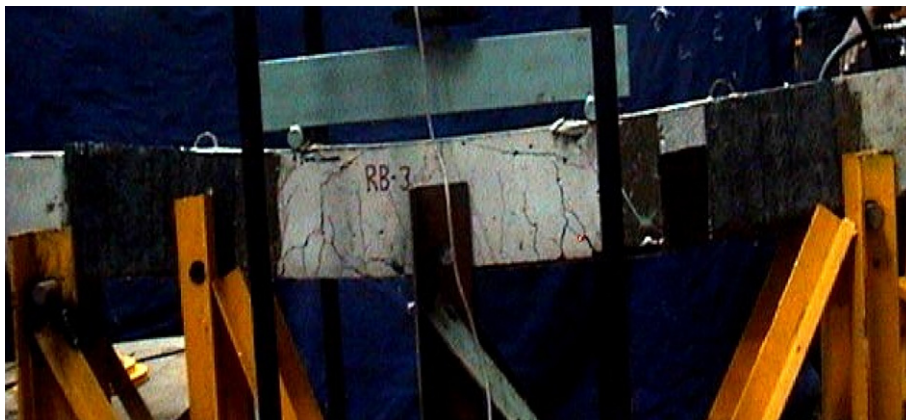
Fig. 7. Beam at failure.
